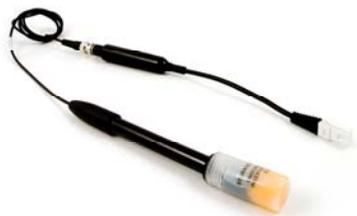
The Tris-Compatible Flat pH Sensor measures the pH of a solution or semisolid. Because the glass membrane is flat instead of a bulb, it is more durable, easier to clean, and allows for flat surface measurements or smaller sample sizes. It features a sealed, gel-filled, double-junction electrode, making it compatible with Tris buffers and solutions containing proteins or sulfides.
